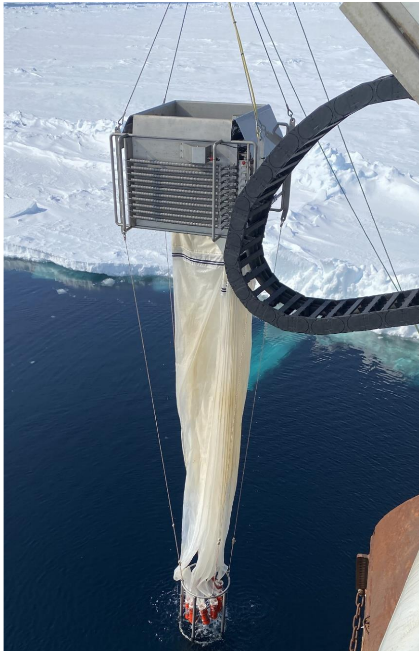
Figure 17. MultiNet Mammoth, sampling capacity: 9 depth strata, opening area: 1 m 2 . Photo: Anette Wold (NPI)
