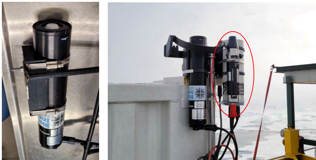
Left: underwater unit. Right RAMSES ACC-VIS irradiance reference radiometer..
