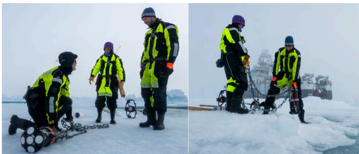
ADCP Signature-500 deployment at Amundsen Sea ice station. Photos: Trine Lise Sviggum Helgerud/NPI
