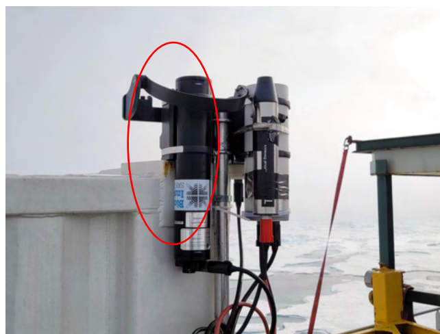
Left panel; RAMSES MRC-VIS radiometer mounted on a floating frame, right panel: RAMSES ACC-VIS irradiance reference radiometer.
