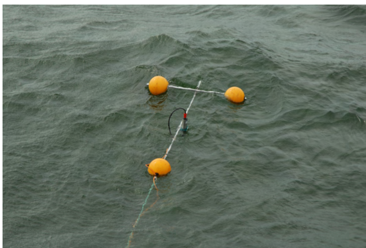
Left panel; RAMSES MRC-VIS radiometer mounted on a floating frame, right panel: RAMSES ACC-VIS irradiance reference radiometer.
